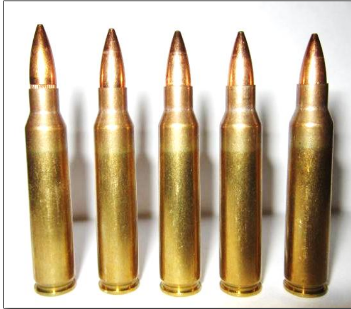
Figure 25: Bullet Setback in Case
